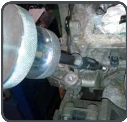
» Glow plug unscrewed, but still stuck in its seat.
