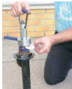
If rod-puller stroke is insufficient: insert one or both spacers (provided) between the support and the clamp in order to further extract the shock absorber rod.
