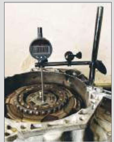
Vertical clearance test with probe extension
