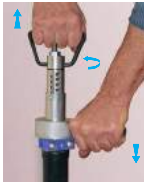
Remove the stem puller and lock it with a slight rotation to the right or left. NB: it is possible to extract the stem by another 20 mm keeping the support still and turning the stem puller.
