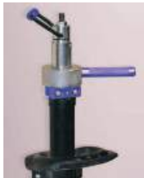
Screw the rod-puller into the support and place the unit on the shock absorber rod. Fasten the shock absorber rod to the rod-puller, using the locking nut.
