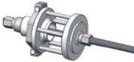
2 Disassembly of the wheel bearing inner ring from the wheel hub
