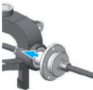
2 Disassembly of the wheel bearing inner ring from the wheel hub
