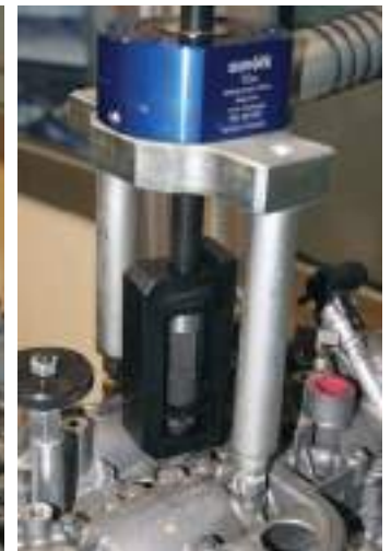
Extraction with GO1015 12T mechadraulic cylinder (optional)
