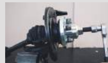
Pushing out the drive shaft, mechanically on the work bench
