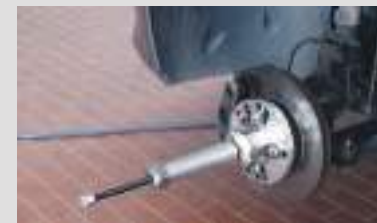
Pushing out the drive shaft, using a 16-Ton Mehadraulic-Spindle, optional code GO1016
