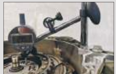
Checking the height clearance of the DSG clutch
