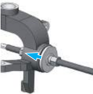
4 Assembly of the new wheel bearing in the axle body
