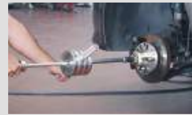
Pulling out the wheel hub, using a slide hammer, optional code GO520
