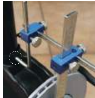
Unscrew the fixing bolt from the disc and mount the wheel alignment tool on the opposite hub wheel.
