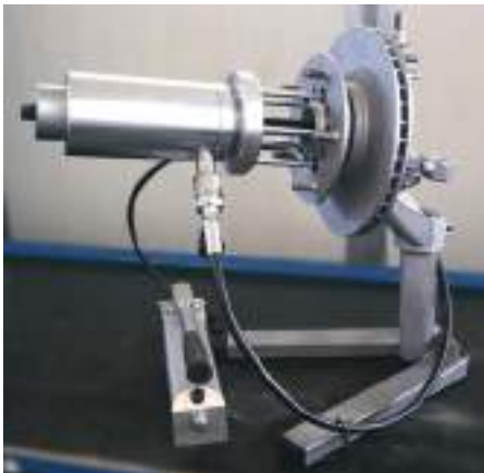
Dismantling of the wheel bearing - brake disc - wheel hubs - change the brake disc.
