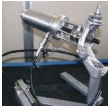
Dismantling of the wheel bearing on the vehicle - changing of the wheel bearing
