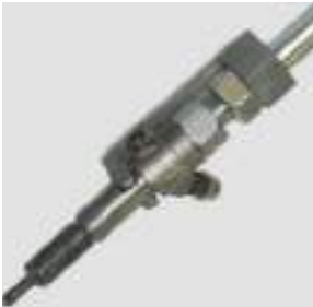
Diesel injector removal
