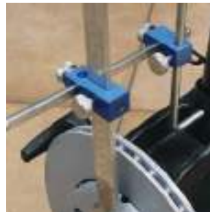
Adjust the pointing measuring tool against the fixing shock-absorber seat.
