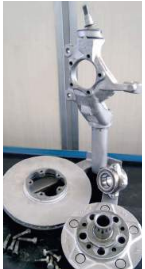
Dismantling of the wheel bearing on the vehicle - changing of the wheel bearing
