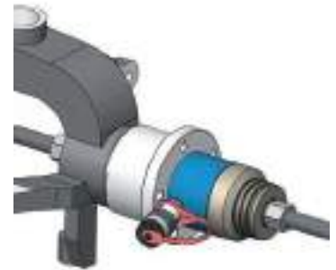
3 Disassembly of the old wheel bearing from the axle body
